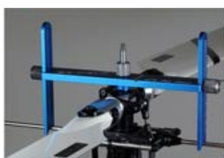
Elevated RC Flybar Lock and Swashplate Level Works GREAT on the 700!!
